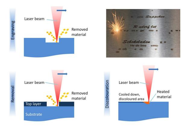
Dependant on the material laser marking is performed with different process technologies.
